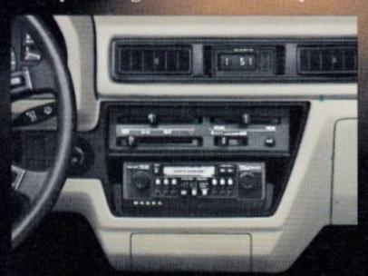
The Prelude's specialized air conditioning is designed to be an integral part of the heating and ventilation system. It has a 3-speed blower, and fully adjustable outlets to provide the desired amount and direction of temperature-controlled air.
