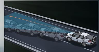
With the new Lane Departure Warning (LDW)<sup>10</sup> system, a small camera between the windshield and the rearview mirror can track lane markings on the road. The system alerts you when it detects you moving into a different lane without signaling (EX-L models).
