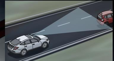
The new Forward Collision Warning (FCW)<sup>9</sup> system can detect the presence of vehicles in front of you and issues alerts when it calculates that you are at risk of a collision (EX-L models).
