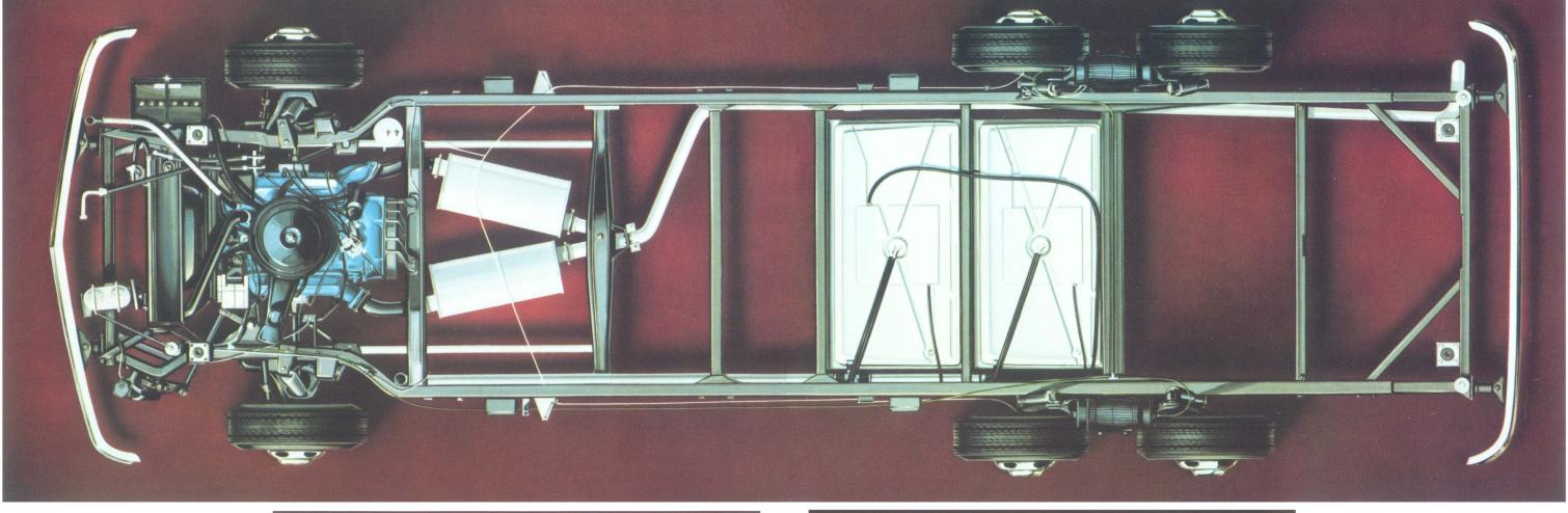
had to fulfill a variety of functions. For example, it had to be able to soak up bumpy roads, as well as cruise the Interstate. So, in the rear, you'll find four wheels in tandem. Not dual. Suspended on air, not stiff steel springs. This happy combination smooths the ride and produces a wide stance.
