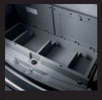
The rear cargo convenience centre is integrated into the rear cargo area behind the third-row seat on EWB models, providing additional storage space for smaller objects. One of the compartments is water-resistant, to hold wet gear.
