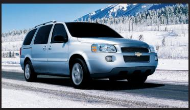
The saying goes that in Canada you can experience all four seasons in a single day. The on-demand Versatrak all-wheel drive adapts to changing conditions automatically, transferring power to the rear wheels when front-wheel slippage is detected. Available on Uplander EWB LT2.
