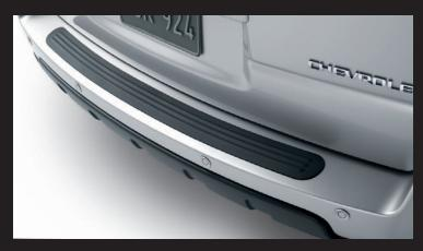
When in 'Reverse', Uplander's available ultrasonic rear parking assist detects obstacles in your path that are at least 25 cm (10 in.) in height. The system then activates audio and LED warnings to alert the driver. Available on Uplander EWB LT2.
