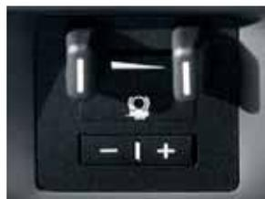
**AN INTEGRATED TRAILER BRAKE CONTROLLER** with instrument panel-mounted control is available on Silverado 1500, 2500HD and 3500HD. Integrated with the ABS, the controller provides immediate and measured brake force signaling to the electric-controlled trailer brake system. Since it's fully integrated with the vehicle's ABS and electric system, there is no requirement for external and/or aftermarket brake control systems.
