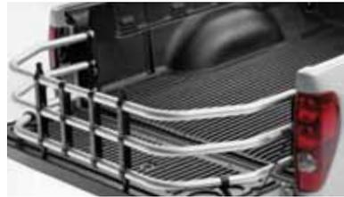
Stretch the capabilities of your Canyon even further. Compatible with GMC Accessory bedliners and tonneau covers, it swings out to create additional functional length for your cargo area, or swings in to create a contained area for smaller objects that need to be secured.
