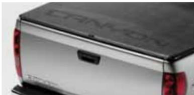
To cover your contents and protect your privacy, this tonneau cover securely attaches to an aluminum frame designed for your Canyon's bed. An ingenious clamping system lets you open the tailgate with the cover in place for greater convenience and easy loading.
