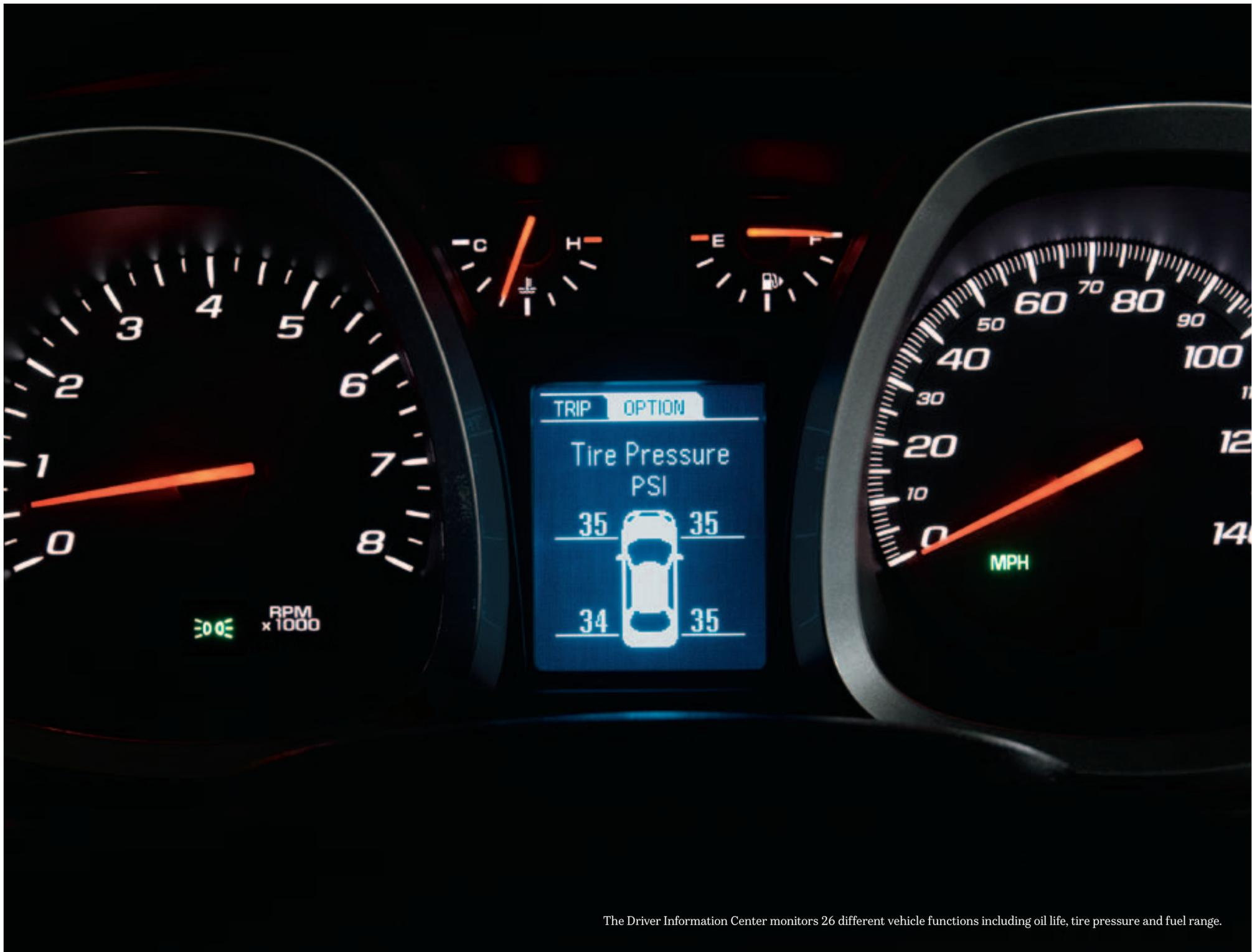
The Driver Information Center monitors 26 different vehicle functions including oil life, tire pressure and fuel range.
