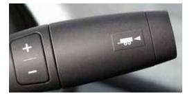
TOW/HAUL MODE To give you even more power to accelerate when trailering or hauling heavy loads, Tow/Haul mode raises transmission upshift points. This feature also helps you slow Sierra by raising downshift points, which use engine compression to slow your Sierra instead of merely braking.
