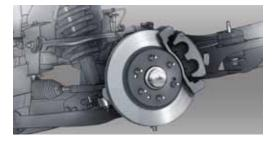
HILL START ASSIST Sensors automatically detect when Sierra is on a 5 percent grade or more. It holds the brakes for up to 1.5 seconds or until the accelerator is pressed, preventing rollback. It is most effective when trailering, giving you time to switch from the brake to the accelerator without rolling.
