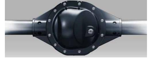
DISTRIBUTION OF POWER Sierra's increased horsepower and torque call for an enhanced way to transmit that power to the pavement. That's why the rear axle features a larger (9.5-inch) ring gear on the V-8s, and the redesigned rear axles are now stronger and beefier to handle the increased power capacity. This robust axle design also provides improved durability.
