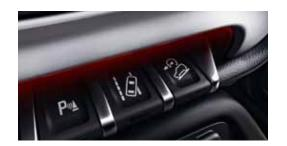
HILL DESCENT CONTROL Activated by pushing a button within easy reach on the instrument panel, Hill Descent Control, included on Z71 models, uses antilock braking to provide a smooth and controlled hill descent in rough terrain without you having to touch the brake pedal.
