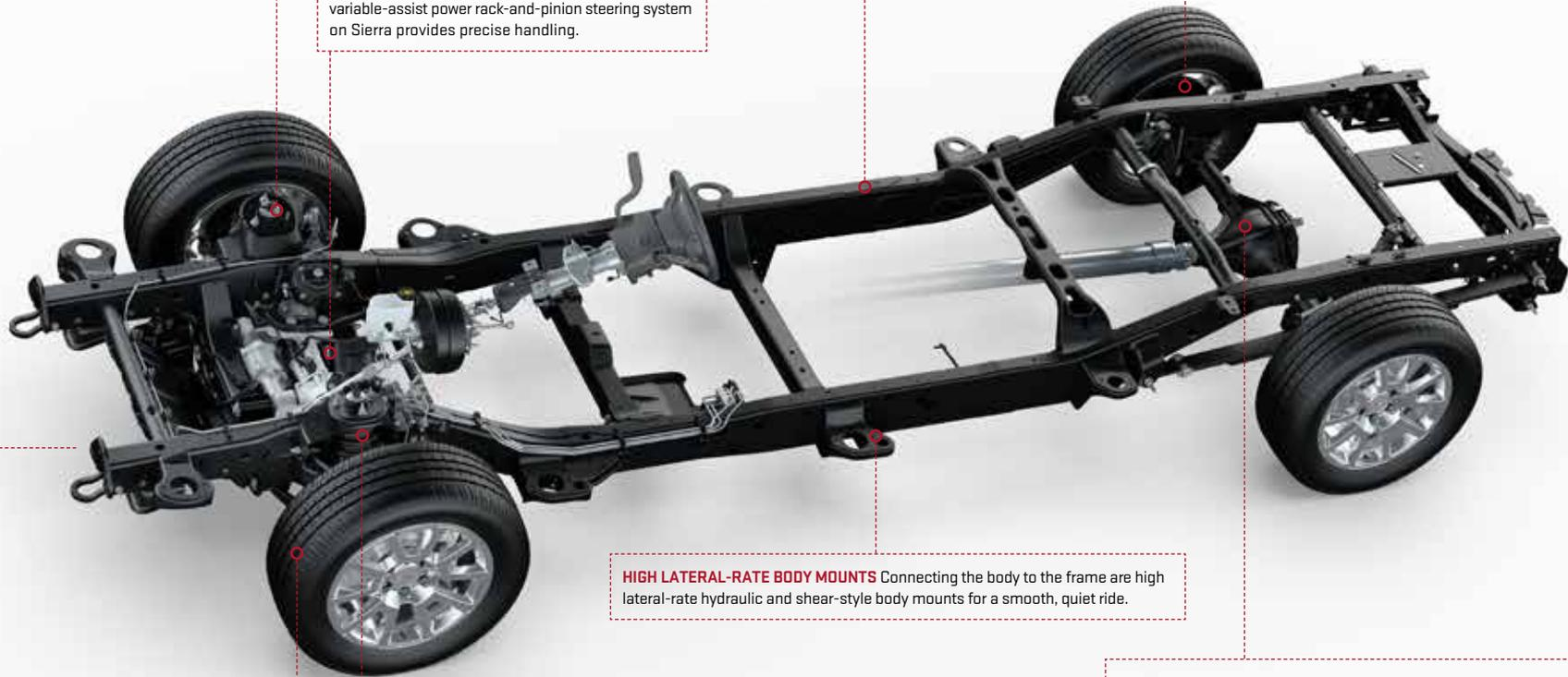
**HIGH LATERAL-RATE BODY MOUNTS** Connecting the body to the frame are high lateral-rate hydraulic and shear-style body mounts for a smooth, quiet ride.
