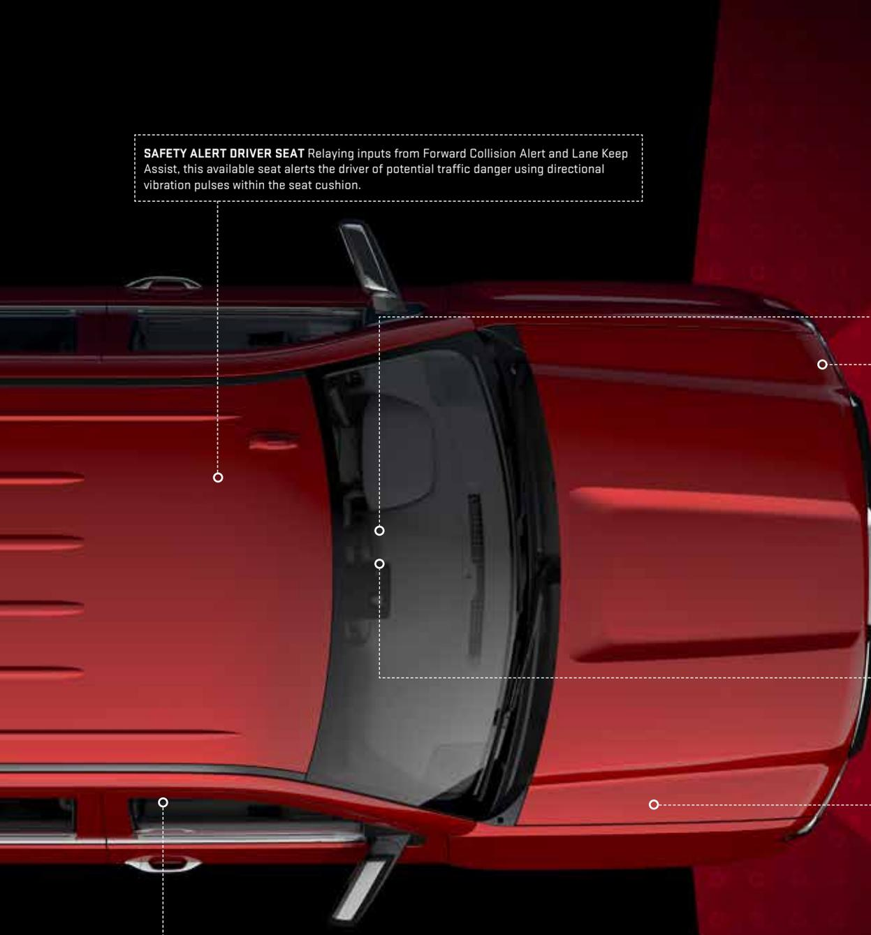
**SAFETY ALERT DRIVER SEAT** Relaying inputs from Forward Collision Alert and Lane Keep Assist, this available seat alerts the driver of potential traffic danger using directional vibration pulses within the seat cushion.
