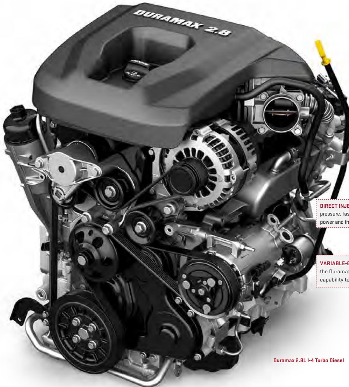
**DURAMAX 2.8L I-4 TURBO DIESEL** The available Duramax 2.8L I-4 Turbo Diesel packs 181 hp at 3400 rpm and 369 lb-ft of torque at 2000 rpm. It's B20 biodiesel capable and mated to a 6-speed automatic transmission that features a Centrifugal Pendulum Vibration Absorber (CPVA) in the torque converter designed to control vibration and noise. When this absorbing damper is energized, it helps to cancel out the Duramax diesel's torsional vibrations.
