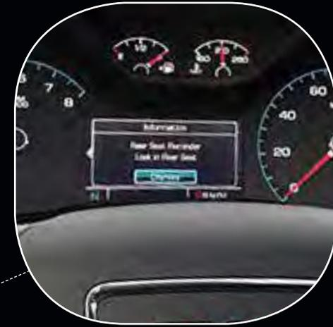
**REAR-SEAT REMINDER** This new feature activates when the rear doors are opened and closed up to 10 minutes before a trip or anytime while your vehicle is on. When Canyon is turned off, an audible alert and a message in the Driver Information Center remind you to check the second row.<sup>2</sup>
