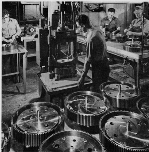
In the government-owned plant at Chevrolet-Saginaw Transmission, planet carriers for the Walker Bulldog tank transmission are being produced at the scheduled rate. Almost completed, these parts are having two holes bored and reamed while burring operations progress in the background.
