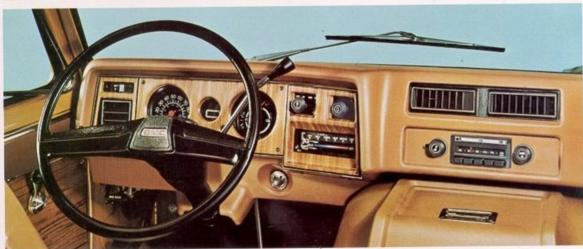
The cockpit-styled Rally dash accommodates the available integral front air conditioning unit with directional controls. A recirculating rear air conditioning unit with separate controls is also available in conjunction with available front dash air.
