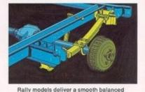
ride with two-stage, multi-leaf rear springs. Two-stage springs, with rubber bushings, provide added support when loaded and a soft ride when empty. Standard spring design features an eight leaf assembly for higher GVW ratings.
