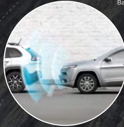
**PARKSENSE<sup>®</sup> FRONT AND REAR PARK ASSIST SYSTEM<sup>4</sup>** Works in tandem with ParkView<sup>®</sup> Rear Back-Up Camera<sup>4</sup> to display previously hidden objects, bringing them to your attention on-screen and with an audible warning so you have time to react. When in Reverse, the on-screen image includes a dynamic distance grid to help gauge your rear perimeter. Available.
