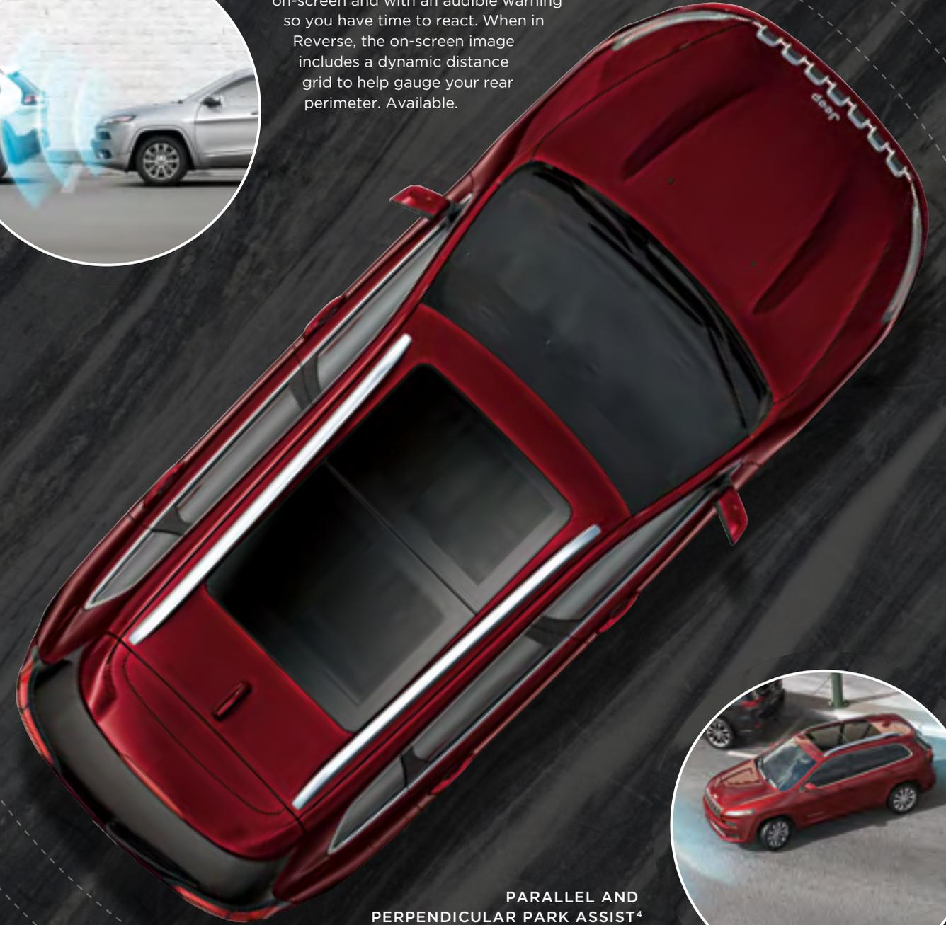
**PARALLEL AND PERPENDICULAR PARK ASSIST<sup>4</sup>** This active guidance system controls steering automatically using ultrasonic sensors that help you ease into parking spots. Includes ParkSense<sup>®</sup> Front and Rear Park Assist<sup>4</sup> sensors. Available.
