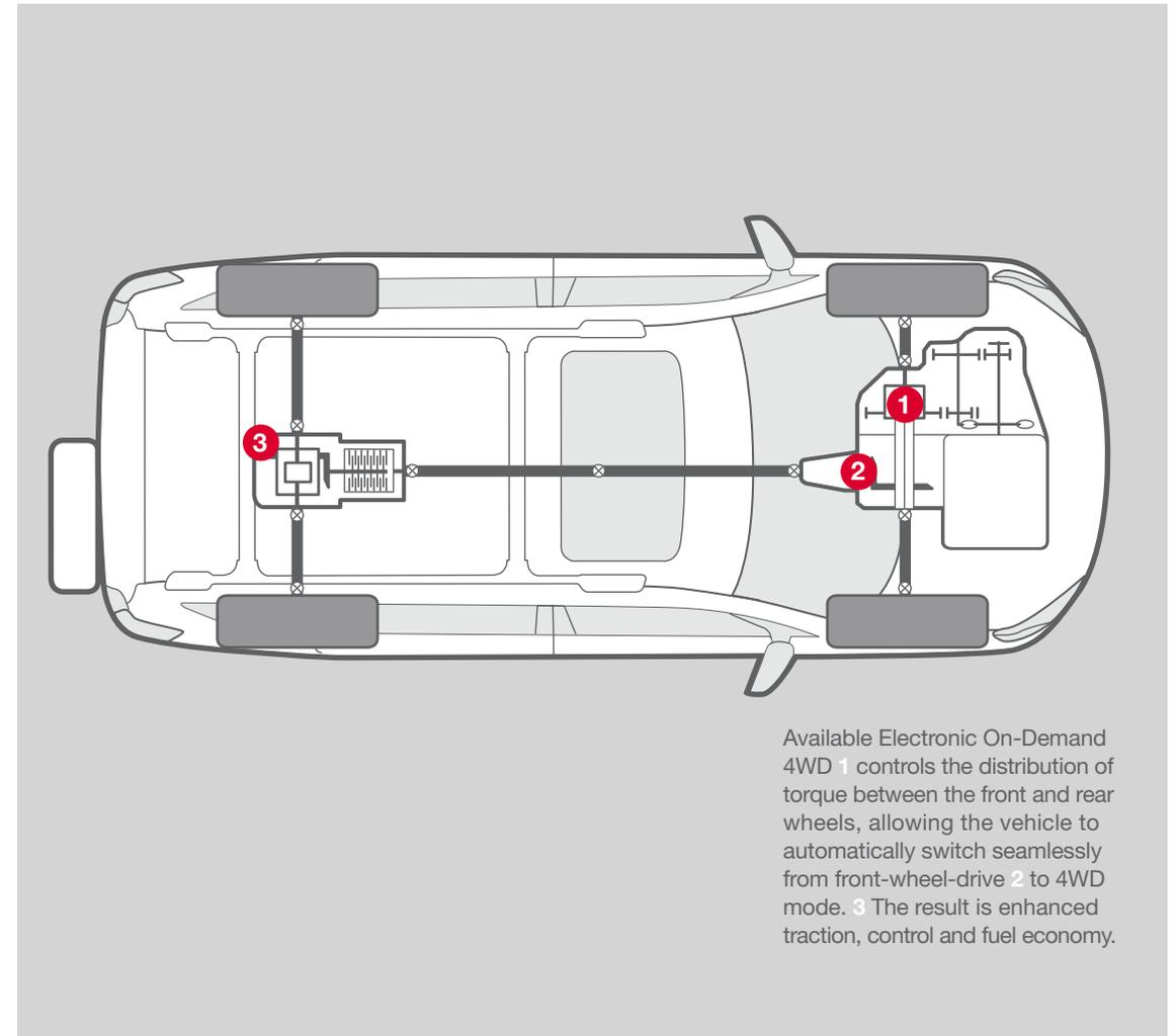
Available Electronic On-Demand 4WD **1** controls the distribution of torque between the front and rear wheels, allowing the vehicle to automatically switch seamlessly from front-wheel-drive **2** to 4WD mode. **3** The result is enhanced traction, control and fuel economy.
