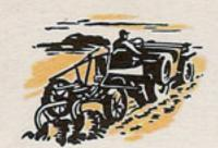
PLOWING. The Universal 'Jeep' operates pulltype and hydraulic-lift implements—has power and traction for field work, with low speeds of 21/2 to 7 mph.
