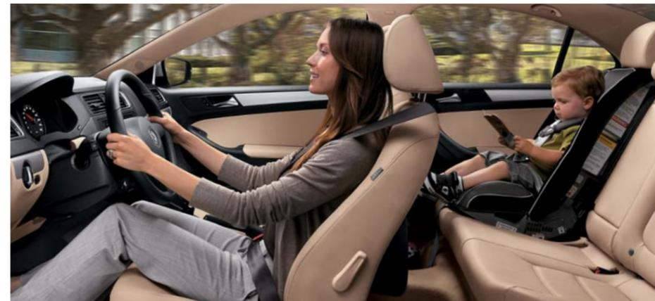
**LATCH (Lower Anchors and Tethers for Children).** Approved by the federal government, LATCH is not only the standard child seat attachment system, but it's standard in all Volkswagen models as well. It allows you to add LATCH-compatible child seats to your VW using built-in anchors that make it easier to install your child seats securely. So whether you already have children, or they're still in your future, your VW is prepared for them.
