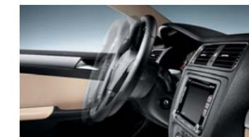
**Telescopic steering wheel.** Using the tilt function to properly adjust the steering wheel places the airbag in a more optimized position. Plus, the steering column is designed to collapse on impact, so the airbag has room to create a cushion between you and the dash.
