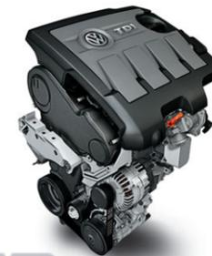
**01 2.0L TDI Clean Diesel engine.** Paired with a 6-speed DSG® performance transmission with Tiptronic® and Sport mode, this 140-hp engine goes up to 565 miles on a single tank.\*\* Yet another excuse to take that road trip you've been wanting.
