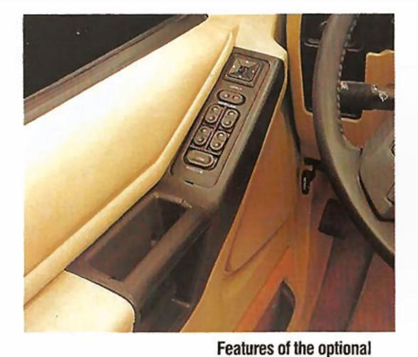
power equipment group (power door locks, windows, and electric remote-control mirrors) are located on a special ergonomic doormounted panel. Tactile controls, easily identified by touch alone, are designed with a "bump" at one end ("on") and a "dimple" at the other end ("off").
