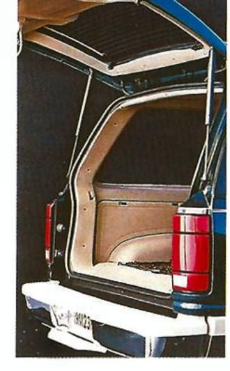
You can access Explorer's spacious cargo compartment from the rear by raising the entire steel liftgate or just the window. Both open with the assist of pneumatic struts. A pulldown handle is included.
