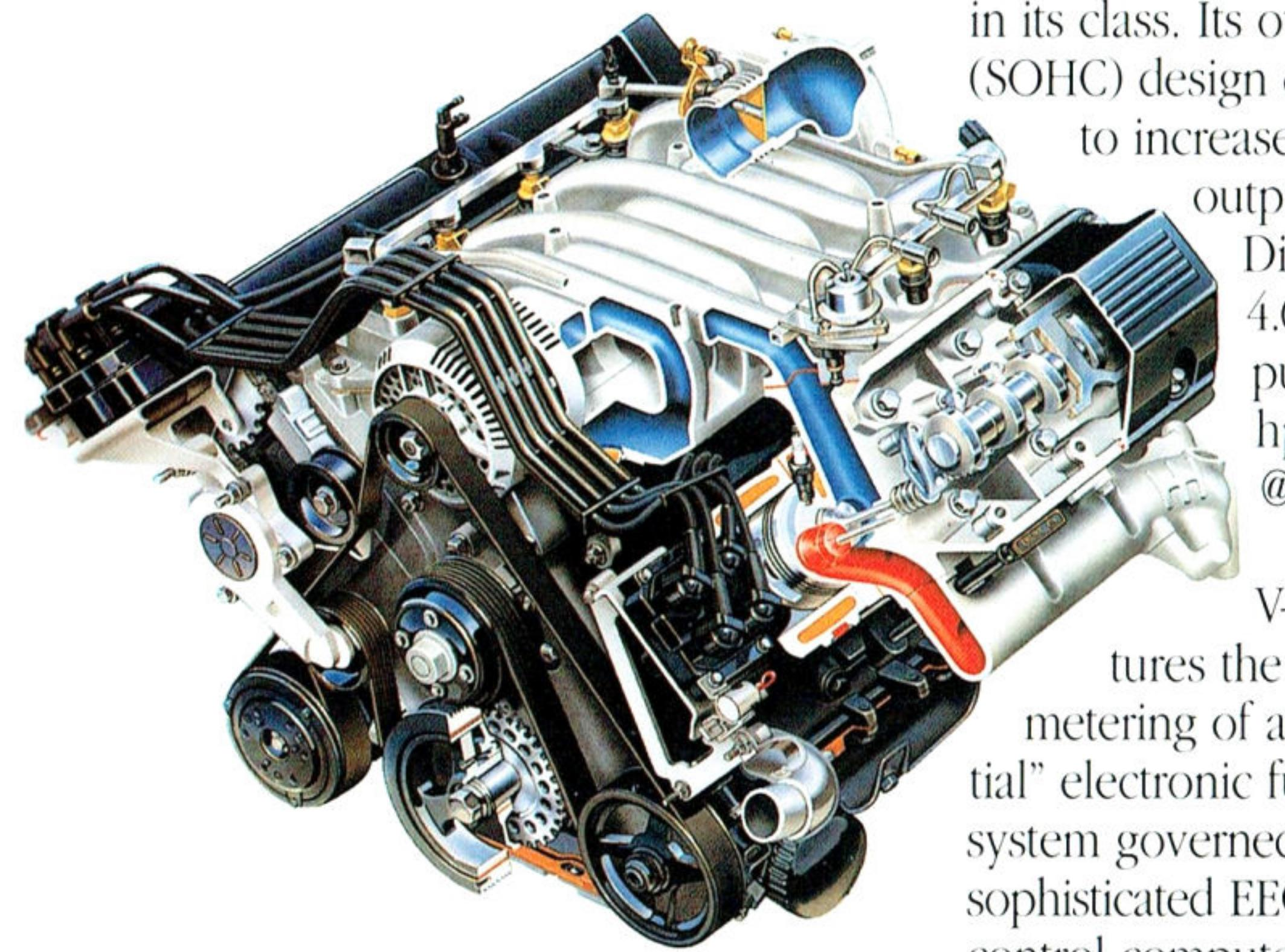
The 4.6-liter V-8 has features such as an overhead cam design and sequential electronic fuel injection. One of the most advanced engines in its class, it's teamed with the smoothness and precision of an electronic 4-speed automatic overdrive transmission.
