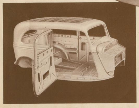
STEEL BODY—The Ford ALL-STEEL body gives greater safety and quiet. It is inherently the strongest, most durable body made. It is not only strong when built but does not deteriorate with age. Its welded one-piece construction assures long life.
