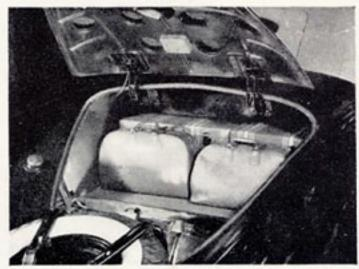
In the rear deck of the Convertible Coupe there is ample room for luggage or sports equipment, as well as the spare wheel. Compartment is dustproof, waterproof, automatically lighted.
