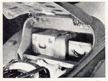
No need for luggage under foot in the Convertible Sedan. This compartment carries it. The spare wheel, which is carried here also, swings out of the way to make loading easy.
