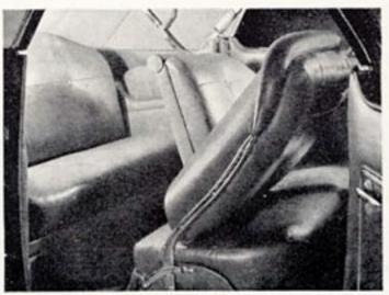
The rear seat of the Convertible Coupe is reached easily through the wide door. The back of the front seat is divided, either half folding forward.
