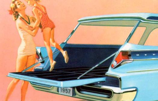
With the liftgate eliminated, the tailgate becomes a convenient “all-clear” loading platform. Now there’s nothing to get in your way when you’re stowing big, bulky objects. Designed to lie flat, and lower by three inches, the new tailgate provides a low “through-level” floor for easier loading and unloading. As for rear opening area . . . it’s over 4 feet wide—and 3¼ feet high. A new “double-action” torsion-bar spring cushions the tailgate going down—provides an assist when you flip-it-up.
