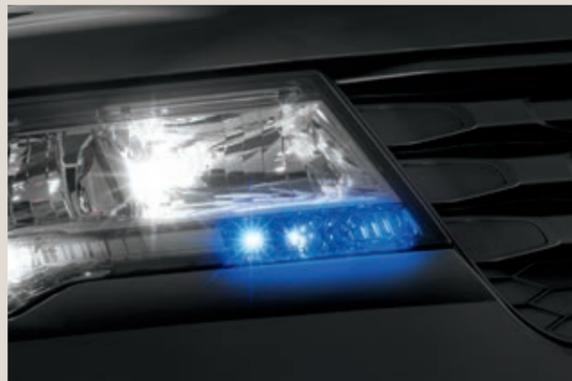
**Forward indicator pocket warning lamps.** Custom-designed, multifunctional Park/Turn/Warn (PTW) LED assemblies integrated into the headlamp system.
