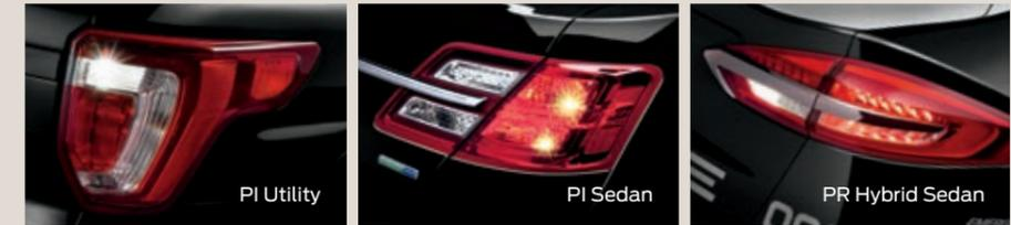
**Police taillamp.** Includes halogen base lamp – plus, for Police Interceptors only, (2) integrated hemispheric lighthead LED side warning lights.
