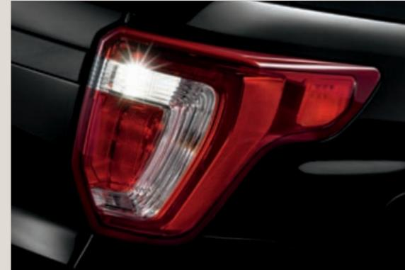
**Police taillamp.** Includes halogen base lamp, plus (2) integrated hemispheric lighthead LED side warning lights.
