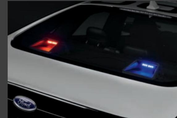
**Police back-window lights.** Includes (2) backlit flashing, linear high-intensity LED lights (driver side red; passenger side blue) mounted inside the decklid. Also comes with **police trunk lights:** (2) backlit flashing, linear high-intensity LED lights (driver side red; passenger side blue) mounted inside the decklid; lights activate when trunk is open.
