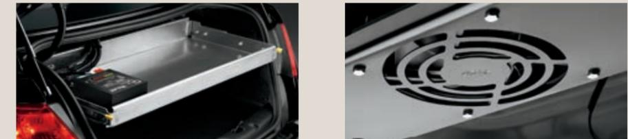
**Trunk electronics tray.** Aluminum, retractable locking tray installed at plant; no height adjustment.
