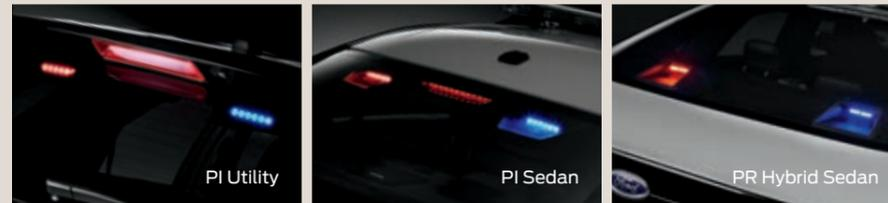
**Police rear lighting.** Includes (2) backlit flashing, linear high-intensity LED lights (driver side red; passenger side blue) with surround cover mounted inside the liftgate glass on the Utility, and inside the back window on the Sedans. Also with (2) backlit flashing, linear high-intensity LED lights mounted inside the liftgate lip on the Utility, and inside the decklid on the Sedans.
