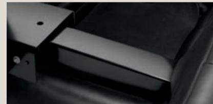
**Rear console plate.** Interfaces with front console mounting plate and extends through 2nd-row occupant area to seat bottom (acting as wiring conduit on top of transmission tunnel).
