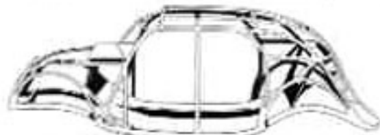
Passenger in Airflow Chrysler ride surrounded by steel girders and all steel body.
