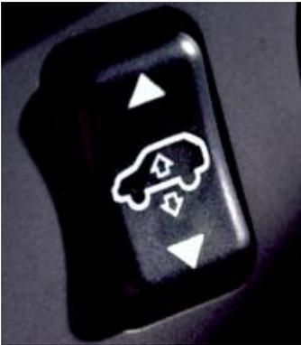
The available Four-Wheel Air Suspension system offers four modes (High, Normal, Low and Access) and can automatically vary its height based on vehicle speed and engine status. For example, the system can provide increased ground clearance one moment and improved aerodynamics for performance driving the next. In some cases, automatically, to help lessen wind resistance. When parked, the RX conveniently assumes its lowest point for easier passenger and cargo loading.
