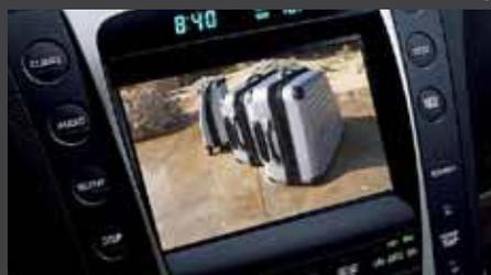
To help you keep an eye on things, the GS features an available small backup camera<sup>19</sup> concealed just above the rear license plate. Place the GS in reverse and the bright, multi-informational color display provides an expanded view of the area behind the vehicle. This allows you to back up with more confidence, so you can quickly get back to doing what the GS does best: moving forward.
