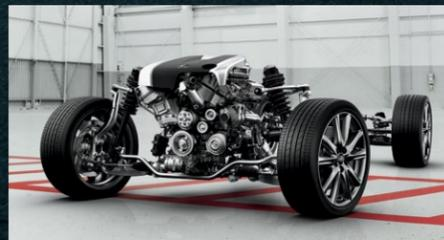
All-new front and rear suspensions were engineered with aluminum components, reducing unsprung weight and delivering significantly greater agility. In the rear, improved suspension geometry further enhances control and tire cornering force. Learn more at [lexus.com/GS/platform](http://lexus.com/GS/platform).
