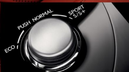
throttle mapping. Available Sport S+ mode goes a step further by also tightening the suspension and increasing steering feel. In both Sport modes, the transmission's shift points are automatically altered coming into and out of corners for sharper acceleration. And during manual gear changes, steering-wheel-mounted paddle shifting is enhanced by precise downshift rev-matching.
