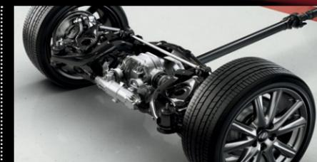
the front for optimal agility and control. At low speeds, the rear wheels turn in the opposite direction for precise maneuvering and a tighter turning circle. All the while, the Variable Gear-Ratio Steering (VGRS) system provides optimized responsiveness and a more direct steering feel.
