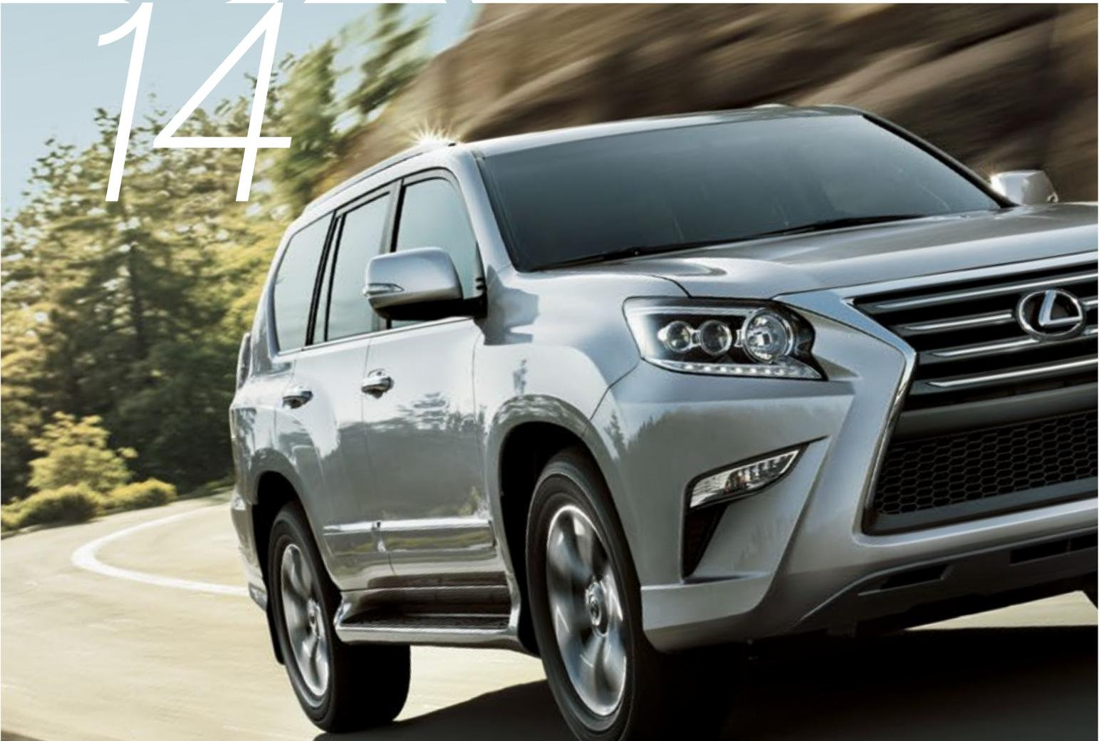
**GX 460** 301-hp<sup>1</sup> 4.6-liter V8; dual Variable Valve Timing with intelligence (VVT-i); six-speed automatic Electronically Controlled Transmission with intelligence (ECT-i); full-time four-wheel drive (4WD); seven-passenger seating.
