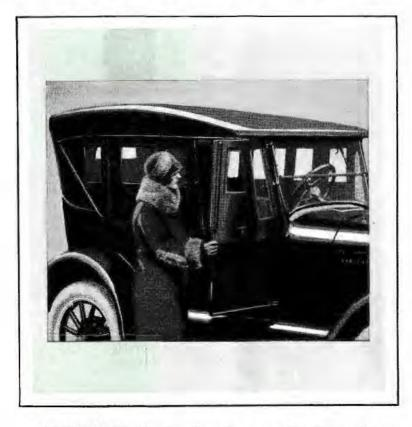
TOURING Car has four doors, making it easy for passengers to enter and leave. Close-fitting curtains open with the four doors and make the car practical and comfortable in cold or stormy weather. The light, strong top may be quickly lowered or raised for summer touring or sport usage.
