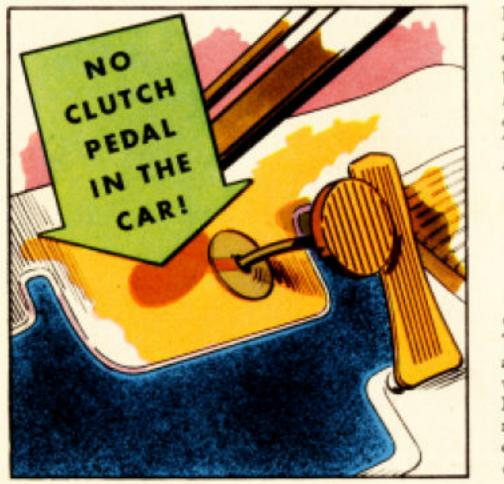
Hydra-Matic Drive's exclusive combination of a fluid coupling and a fully automatic transmission takes the place of the conventional clutch mechanism entirely. All the functions ordinarily performed by a friction-type, foot-operated clutch are taken care of automatically with Hydra-Matic Drive. This means there are no conventional clutch facings to wear out . . . and to be adjusted. There's no clutch pressing for the driver to do. There's not even a clutch pedal in the car.
