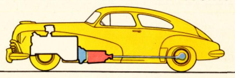
Directly behind the engine in a car equipped with Hydra-Matic Drive is a modern, high efficiency fluid coupling, shown in blue in the diagram above. The driving force from the engine is conveyed through this hydraulic unit of whirling oil, which gives a "cushioning effect"—a smoother, more flexible flow of power to the rear wheels . . . But that's only half the story.
