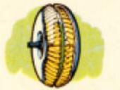
One important part of Hydra-Matic Drive is its fluid coupling, a cushion of oil between engine and driving mechanism.
