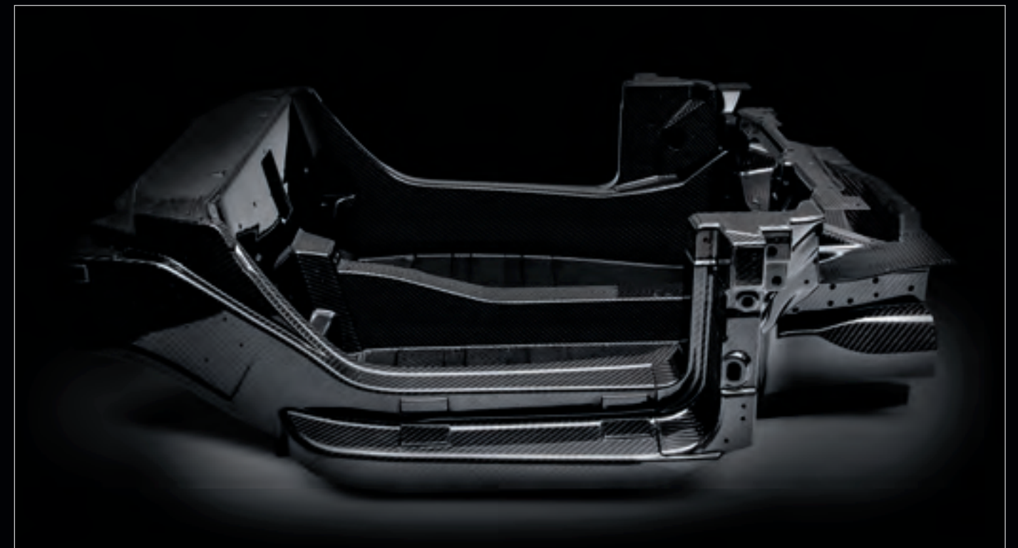
Genuine carbon fiber monocoque chassis
