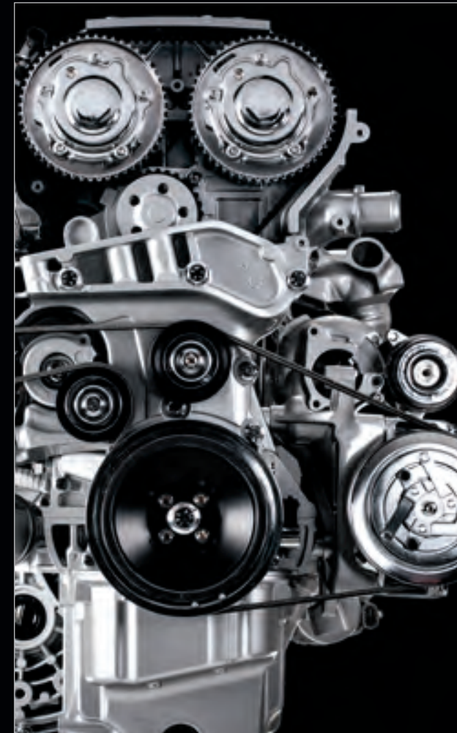
1750 turbocharged, aluminum, 4-cylinder engine
