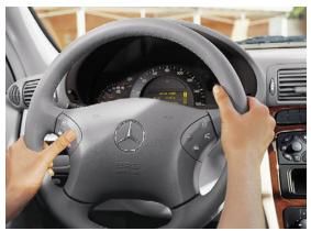
Controls on the steering wheel and a multifunction display let you adjust audio volume and program vehicle settings. You can also check coolant temperature, engine oil level, trip computer data and more – even the distance to the next service as calculated by the clever Flexible Service System.
