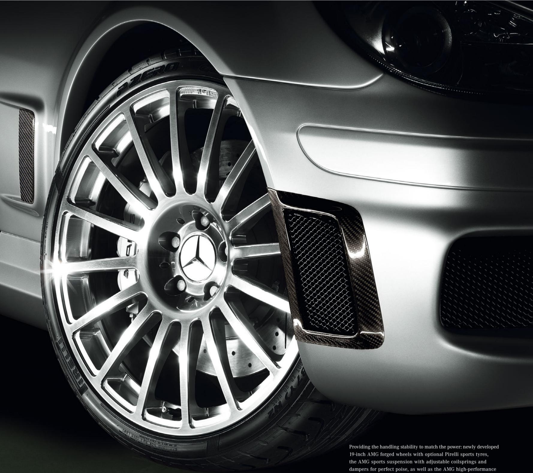
Providing the handling stability to match the power: newly developed 19-inch AMG forged wheels with optional Pirelli sports tyres, the AMG sports suspension with adjustable coil springs and dampers for perfect poise, as well as the AMG high-performance braking system with 6-piston callipers and 360-mm composite brake discs at the front. The front suspension cross-brace means extra strength for enhanced lateral dynamics.
