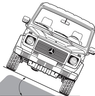
Directionally stable on lateral slopes up to 54 %
