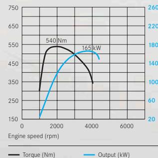
**G 320 CDI.** The 3-litre V6 diesel engine achieves its maximum output of 165 kW (224 hp) at just 3800 rpm
