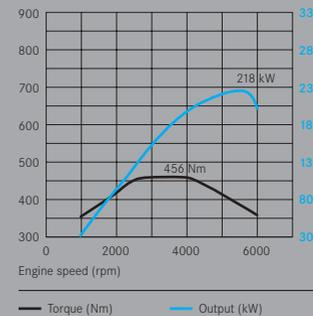
**G 500.** The G 500 achieves its peak torque of 456 Nm across a broad engine speed range from 2800 rpm to 4000 rpm
