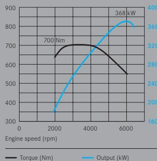
**Full power ahead.** The impressive torque of 700 Nm is available across a broad engine speed range from 2570 rpm to 4000 rpm
