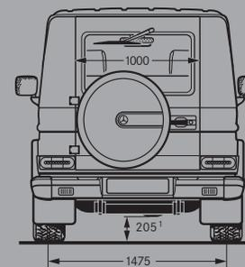
The dimensions shown are mean values (in mm) and apply to standard-specification vehicles carrying three occupants weighing 68 kg each
