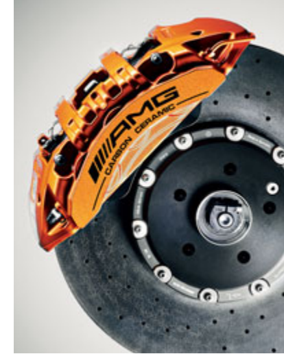
Optional extra AMG ceramic high-performance compound brake system
