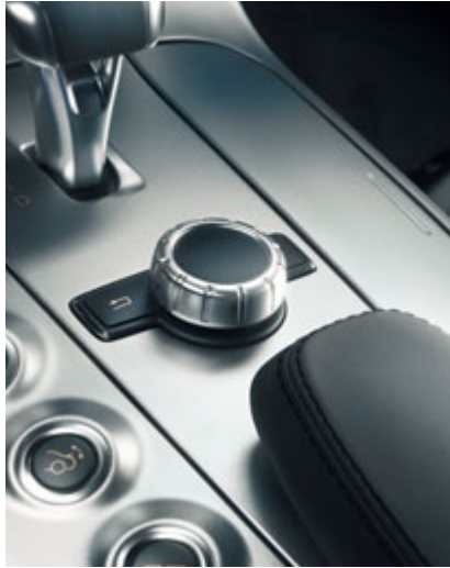
Standard equipment Central control panel for COMAND APS
