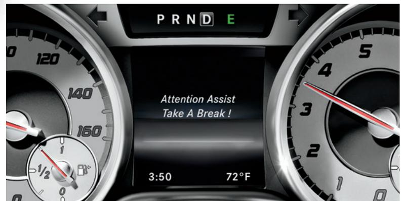
**A watchful eye when it's time for a rest.** ATTENTION ASSIST<sup>®</sup> is a Mercedes-Benz innovation that can alert you if it detects signs of drowsiness on long drives. It measures more than 70 variables, starting in the first minutes of a drive, to establish a pattern. By continually monitoring a variety of driving behaviors along your trip, it can offer a warning tone and encourage taking a rest if it senses you're getting drowsy.<sup>7</sup>
