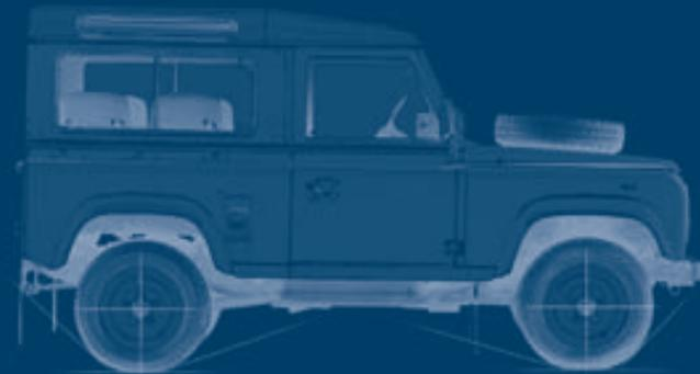
'90' Station Wagon (1984-1990) 1984 Leaf springs upgraded to coil springs. One-piece windscreen introduced. Wind-up front windows replace sliding windows. Polyurethane wheel arches introduced to accommodate wider track.
