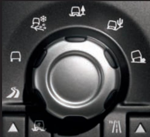
The Terrain Response® system includes Dynamic Program, which gives a sportier, more engaged drive in multitudes of conditions.
