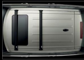
Sports Bars\* VUB502790 Fixed position crossbars, easily removed when not in use. Aerodynamic profile. Load capacity 212.1lbs. Vehicle height when fitted 76.3 inches.
