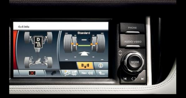
Terrain Response® uses a rotary dial on the center console (and grouped in a convenient cluster with the air suspension height control, Hill Descent Control (HDC®) with Gradient Release Control (GRC) and the High/Low Range selector) to choose settings for different driving environments.
