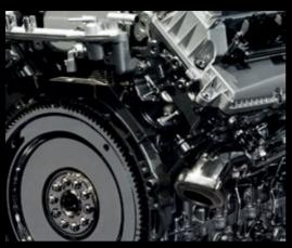
Range Rover engines incorporate Dual Independent Variable Camshaft Timing (DIVCT), which provides increased torque at low speeds and greater power at higher speeds.
