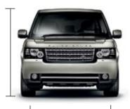
Front wheel track 64.1 inches/1.629mm Height 73.9 inches/1,877mm<sup>†</sup> Standard height includes satellite antenna †Access height air suspension setting reduces height given by 1.6 inches/40mm to 72.3 inches/1,837mm
