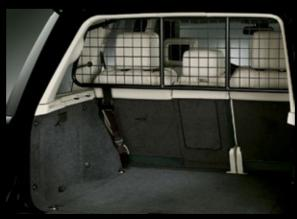
Cargo Barrier Half Height LR007320 Easily removed.
