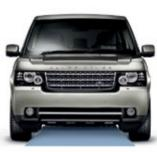
Obstacle Clearance Ground clearance off-road height up to 11.1 inches/283mm, with air suspension raised (Standard ride height 9.1 inches/232mm)
