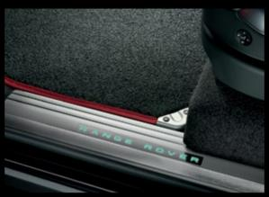
Illuminated Tread Plates VPLMV0063 Illuminates the words Range Rover when the driver or passenger door is opened.
