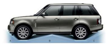
Approach Angle Standard ride height 29° (22.9°)\*, off-road 34° (25.4°)\* to spoiler with air suspension raised
