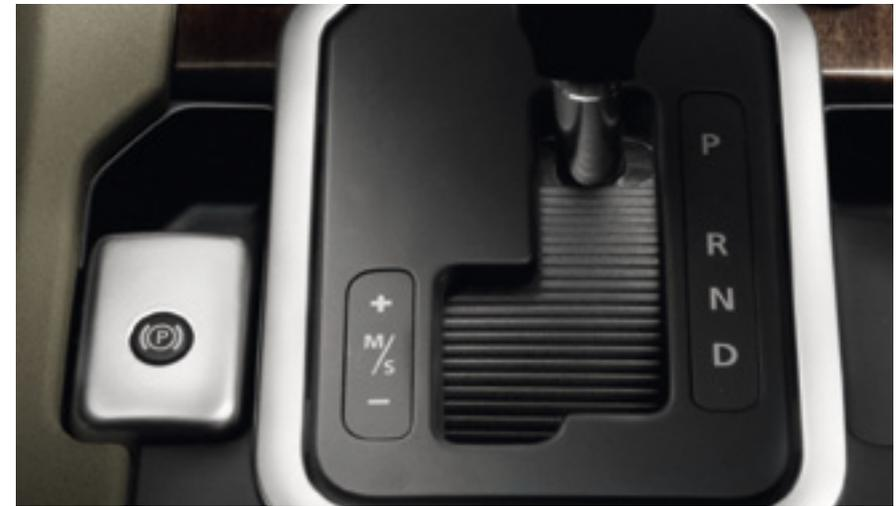
**ELECTRIC PARKING BRAKE (EPB).** A lever is located next to the gear selector to electrically apply and release the parking brakes on the rear wheels. A simple pull of the lever applies the brake manually and a press releases it. The parking brake will also release automatically upon drive away.
