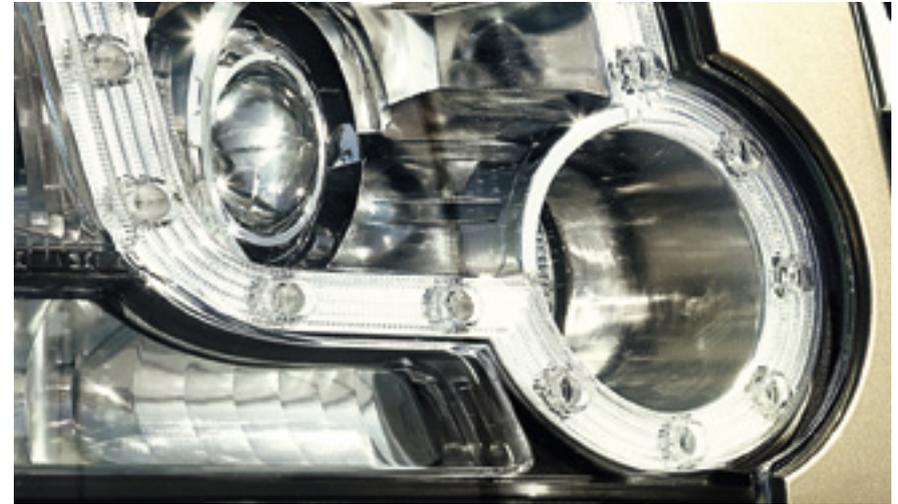
**AUTOMATIC HEADLAMPS WITH HIGH BEAM ASSIST\*.** Detect vehicle headlamps/tail lights and dip the high beam until the light source is out of range. The system is able to distinguish between automotive and non-automotive light sources.
