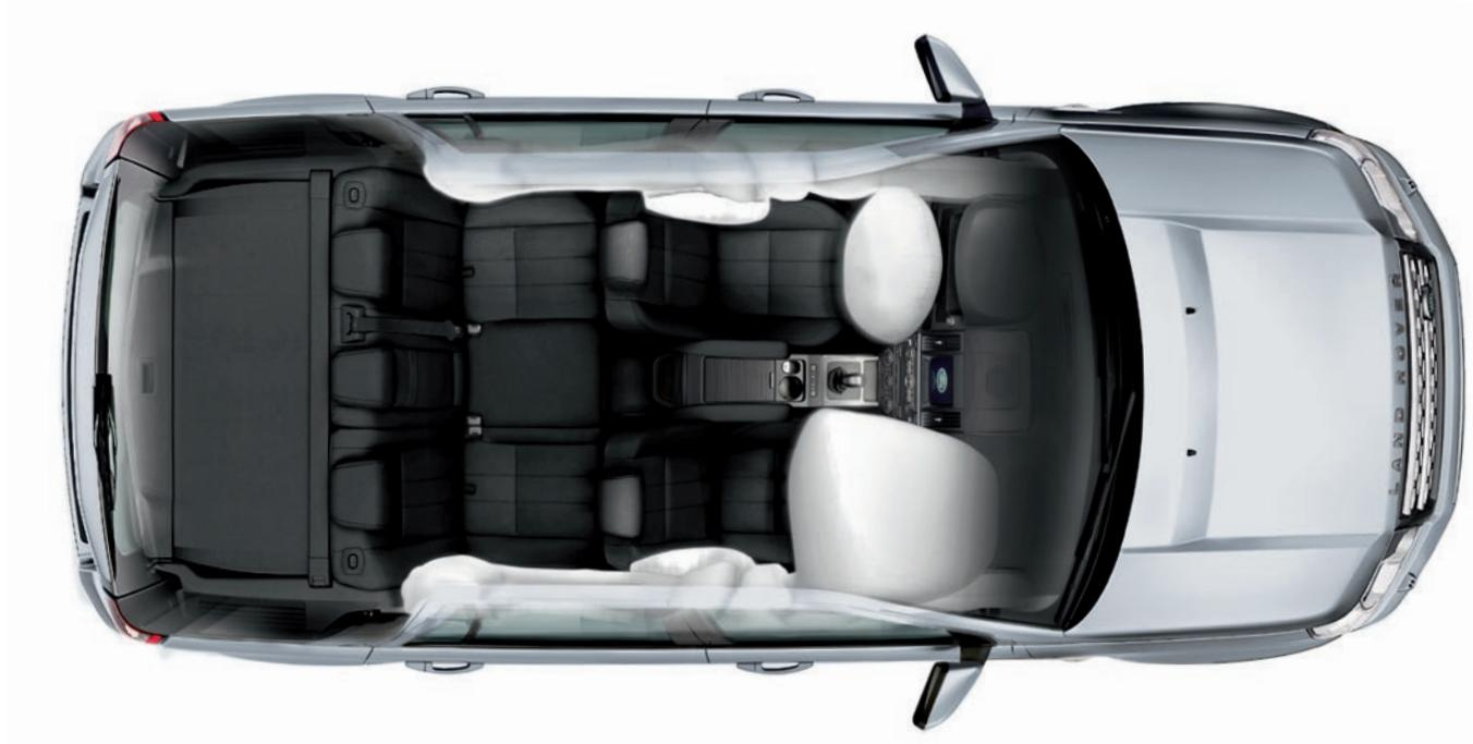
With a raft of safety systems, the Land Rover LR2 has been built to take almost anything life throws at it. Firstly, its strong monocoque body and inner body cell, both of which are protected by crumple zones, are designed to absorb energy on impact.
