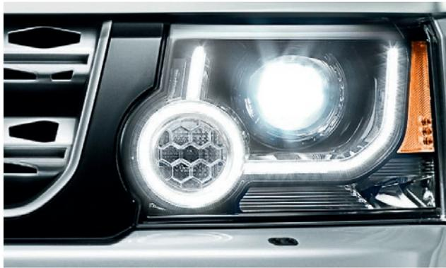
**Automatic headlamps with High Beam Assist and adaptive Xenon headlamps with LED signature\*†**
