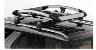
Luggage Carrier<sup>‡</sup> VPLRR0159 Flexible rack system to facilitate roof carrying. Maximum payload 134lbs<sup>4</sup>.
