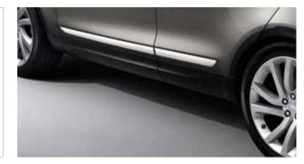
Body Side Moldings VPLRP0286 – Bright finish VPLRP0285 – Black finish (not shown) Enhances the side of your vehicle and provides protection for your door panels from accidental damage by adjacent vehicles.
