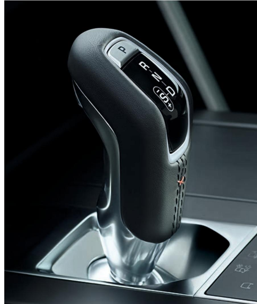
Inside Discovery SVX, a Pistol Shifter adds to the overall enjoyment of the driving experience. Off-road, the Pistol Shifter enables quick and efficient forward and reverse engagement with a simple fore and aft movement. This allows the driver to better negotiate deformable surfaces such as deep snow, sand and mud.
