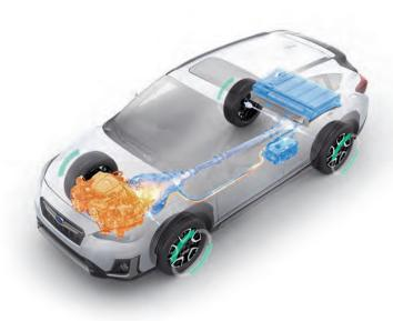
In everyday driving, the system will run on a combination of electric and gas power. It can also recover energy via regenerative braking.
